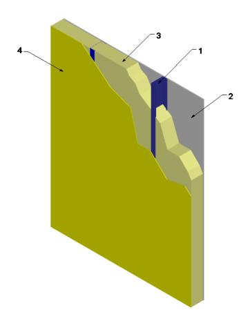
WALL FRAMING: Install 3-5/8 in. deep, 20 GA galvanized steel studs spaced max. 24 in. on center (oc). Secure steel studs to 3-5/8 in. 20 GA top and bottom track (not shown) using #8, 7/16 in. long, self-tapping, pan-head framing screws.
